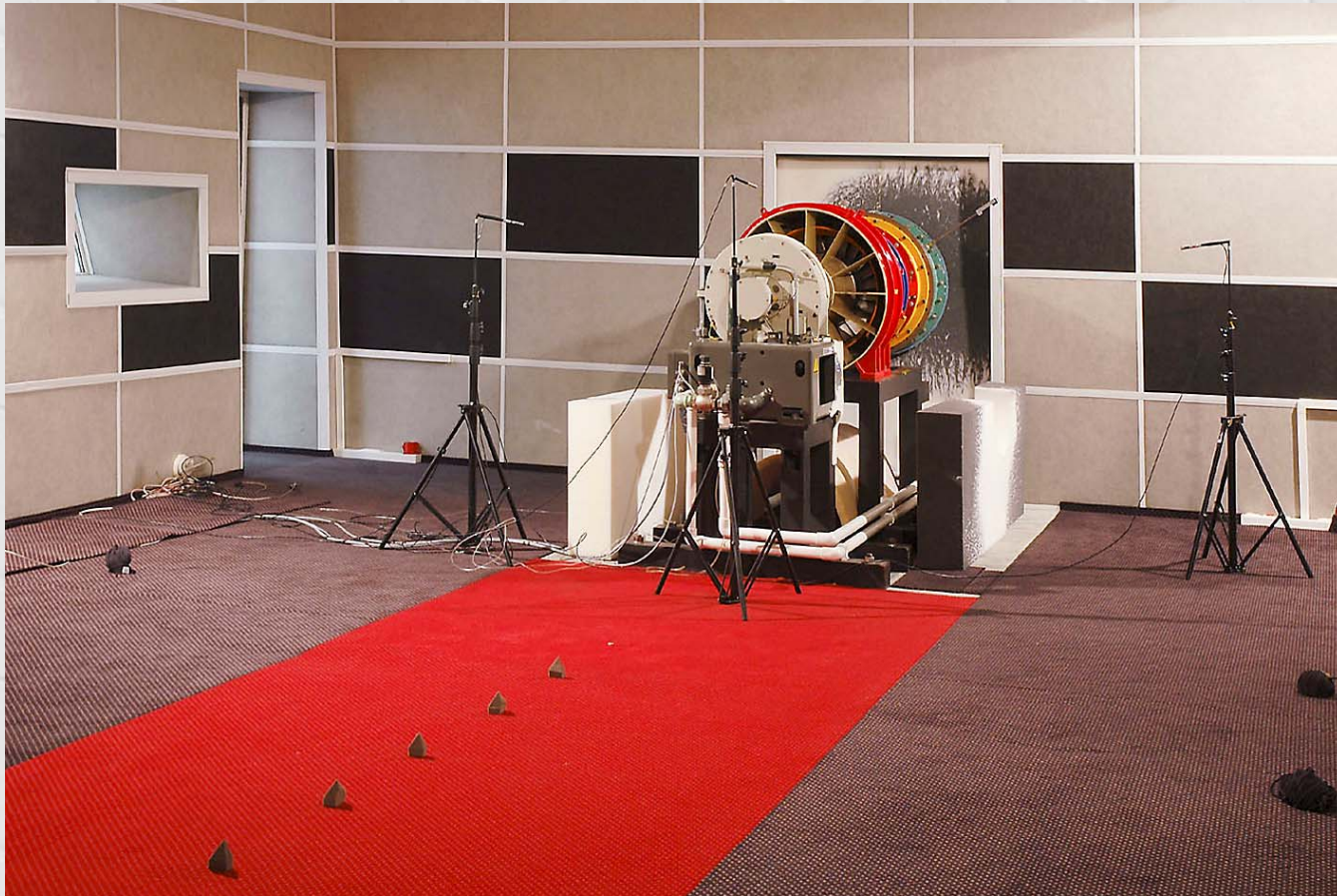
Anechoic chamber for aeroacoustic investigations of turbomachines
