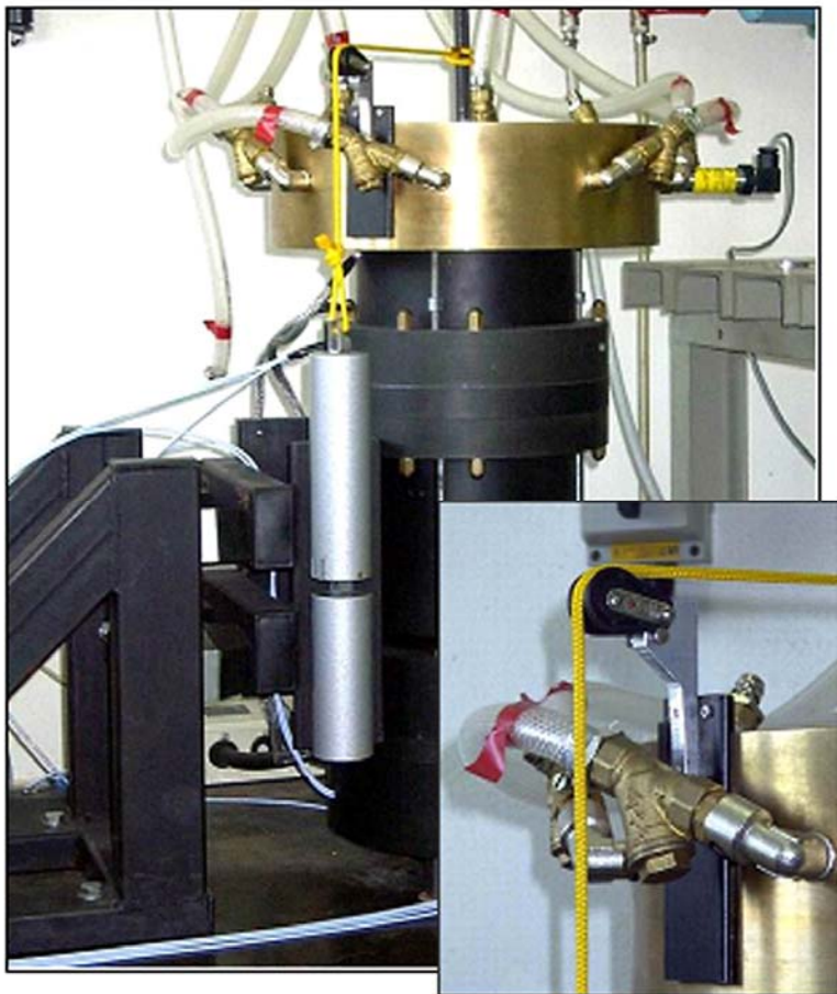
Test stand with a rotor supported in active magnetic bearings for identification of forces in the labyrinth seal
