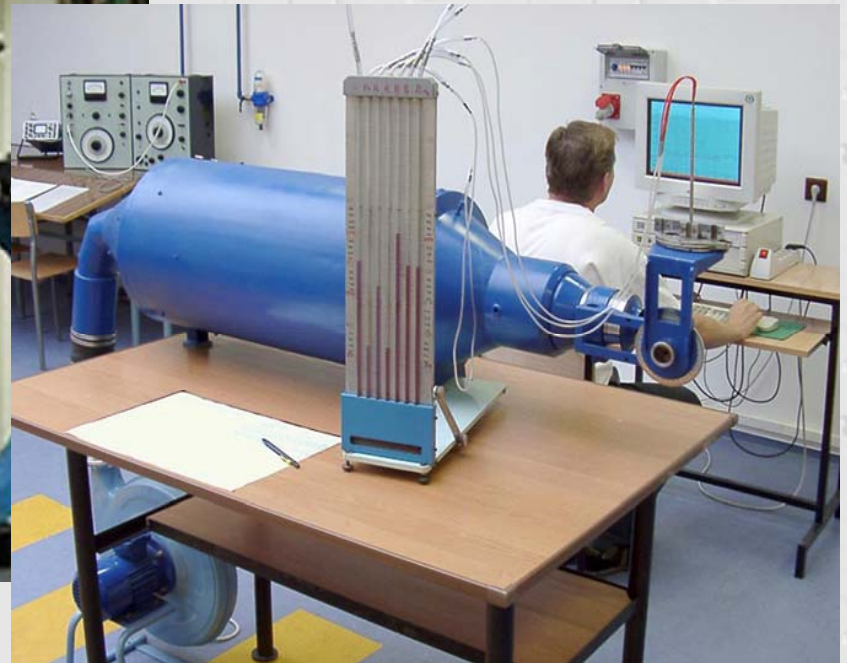
Wind tunnel for investigations of probe properties
